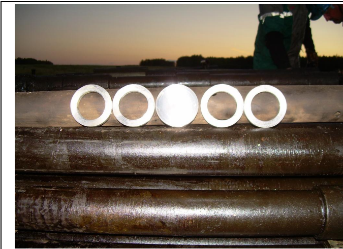
Photo 1. A stopper ring for fixing 15 FCR in vertical position inside PCP
