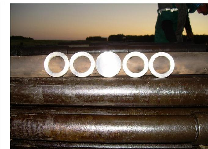
Photo 1. A stopper ring for fixing 15 FCR in vertical position inside PCP
